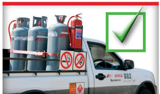
As LPG is heavier than air, any accidental release of gas will sink to the lowest point. Therefore, cylinders should always be **kept away from**:
